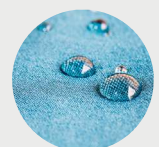
Instead of soaking through, fluids bead up and roll off the fabric.
